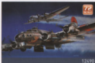
B-17G Another elaboration of the B-17 design, the G sported a chin-mounted turret to fend off oncoming attackers.
