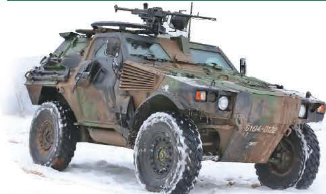
VBL (Light Armored Vehicle) short ch. 7.62 MG
